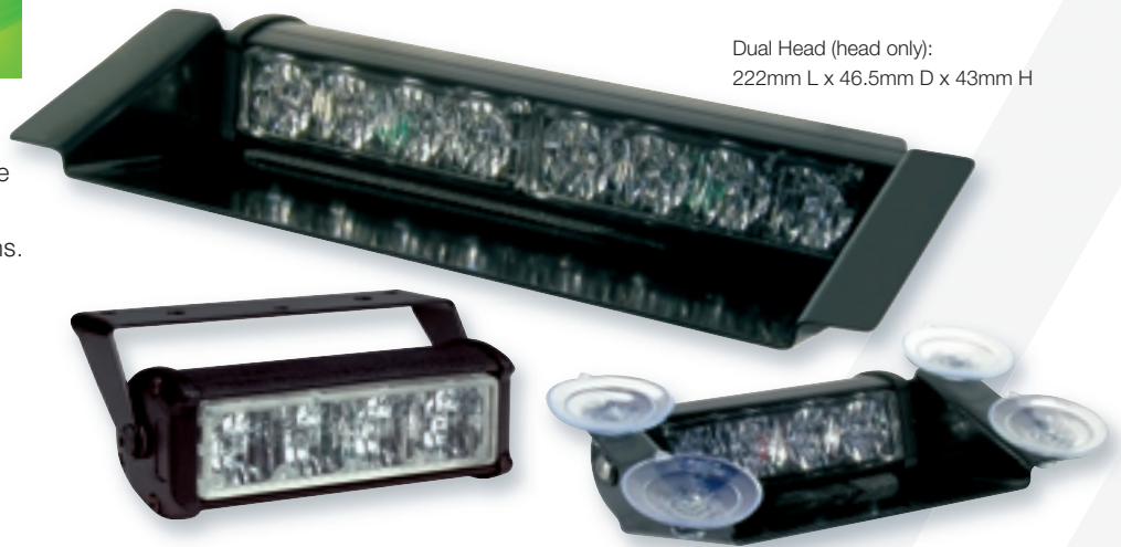
Single Head (head only): 120mm L x 46.5mm D x 43mm H
